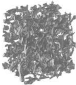
Fig. 1 \mu -CT of porous polyester
