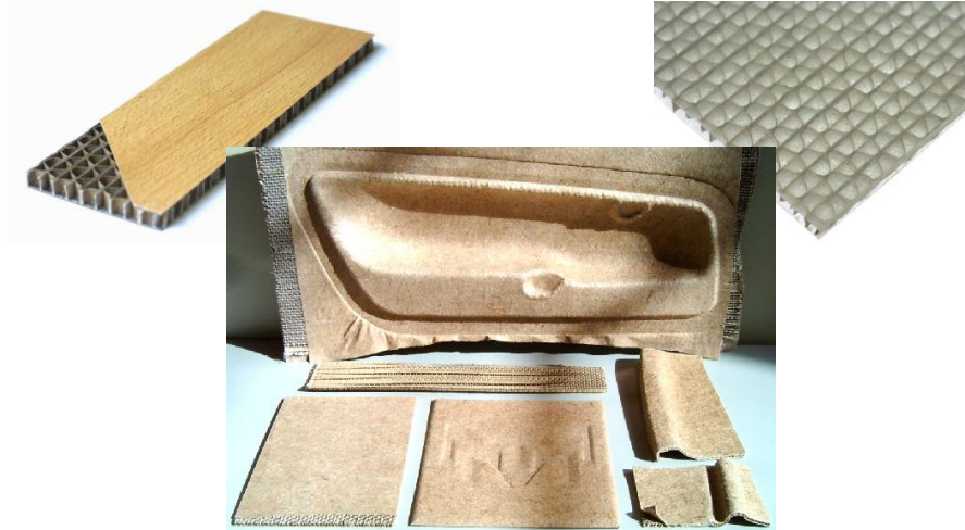
Figure 5. Example of 'Torhex' cardboard honeycombs with natural fibre composite skins, thus yielding a product fully made of natural fibres.
