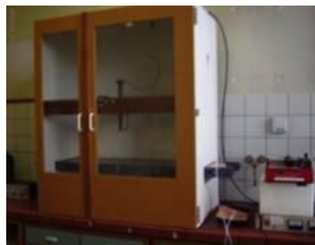
Figure 1- (a) "Needle-printing" electrospinning prototype, (b) concerted movement of both, needle and conveyor belt.
